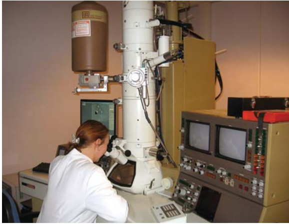
Figure 1.2 Transmission electron microscope. This is a microscope in which the image is formed by electrons transmitted through the specimen. Photograph courtesy of Kathryn Newton.
