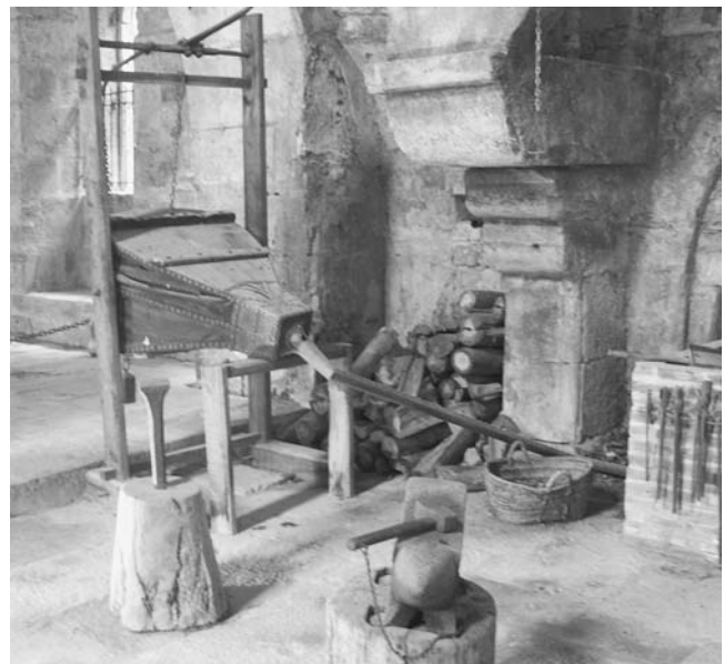
A bellows for metalworking at the abbey of Fontenay in Burgundy (Courtesy Edward English)
