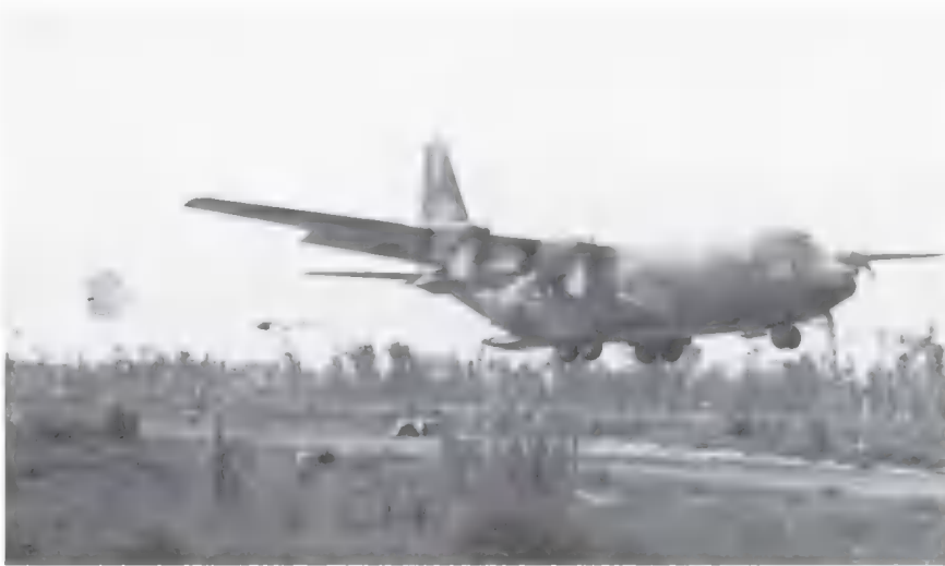
Top: This C-130 Hercules releases its Low-Altitude Pallet-Extraction System (LAPES) load while skimming over the airstrip at Camp Thien Ngon in October 1968. (USAF) Center left: C-7 Caribous, lined up at the Pleiku airfield, await parachute-equipped cargo sleds destined for outlying Special Forces camps during June 1969. (USAF) Center right: Crated livestock were airdropped by cargo parachutes to ensure that distant camps had fresh meat. (Author's Collection) Bottom left: C-7 Caribou Air Force flight engineer Technical Sgt. Armand Lara helps Sgt. First Class Joe H. Vargas don a parachute preparatory to a fuel resupply para-drop over Camp Ha Thanh in September 1969. (USAF) Bottom right: A LAPES-delivered truck is driven off the runway by Staff Sgt. Howard F. Cranford at Camp Thien Ngon in late 1968. (USAF)
